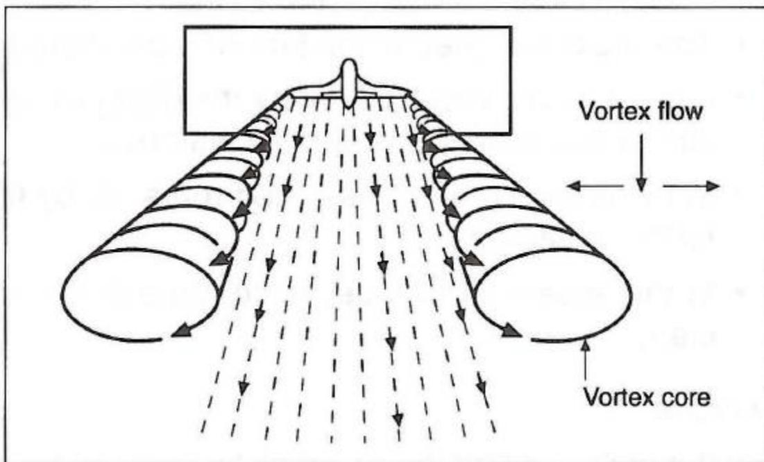
The characteristics of a vortex can be altered by changing the aircraft's configuration. The most intense vortices will be produced by an airplane that is heavy, flying slowly, and with the landing gear and flaps retracted.
