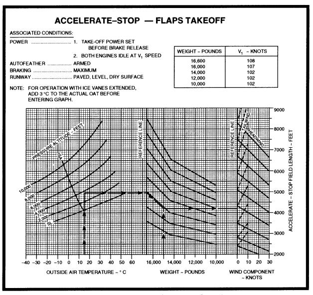
FIGURE 14.—Accelerate-Stop – Flaps Takeoff.
