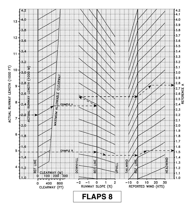
Take-off Weight Limited by Field Length Requirements - All Engines Operating, FLAPS 8
