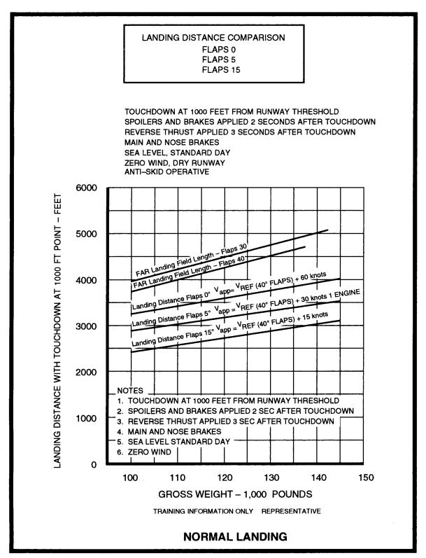
FIGURE 91.—B-727 – Normal Landing Distance Comparison.
